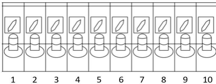
**(1,2) Batt Temp:** Battery Temperature Sensor has no polarity and is needed for voltage correction when using lead acid batteries.
