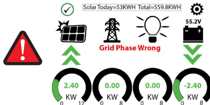
If the Sol-Ark screen shows **Grid Phase Wrong** there is a phasing issue with your wiring and it may cause overload faults (F18, F26, F34) even with the Load breaker **off** and **WILL CAUSE DAMAGE if left unchecked**.
