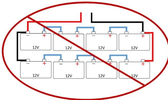
**Do NOT reverse polarity of batteries!**
