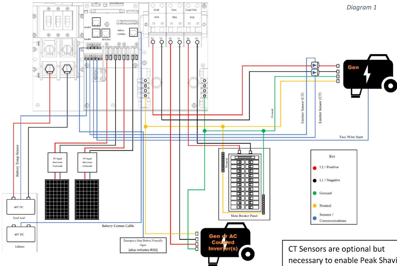
CT Sensors are optional but necessary to enable Peak Shaving. See pg. 21 and pg.39 for additional info.
