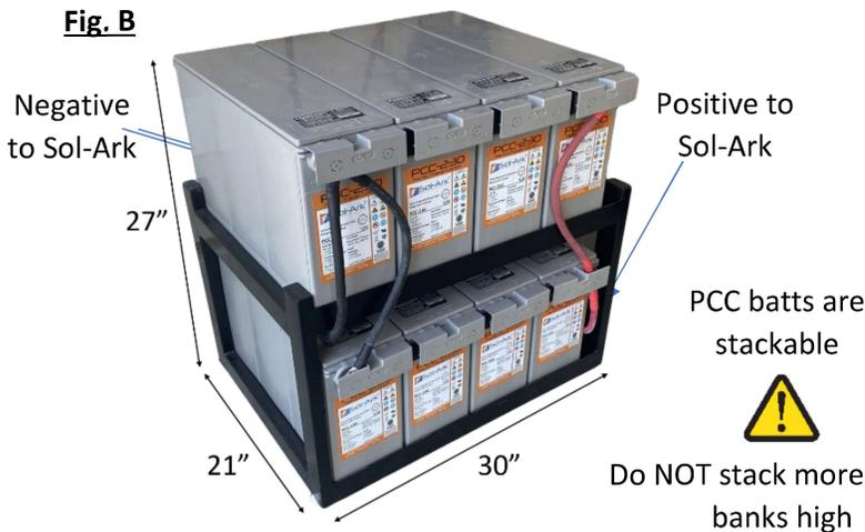
Sol-Ark 12K is a **48V** system. Do NOT wire the battery bank to any other nominal voltage.
